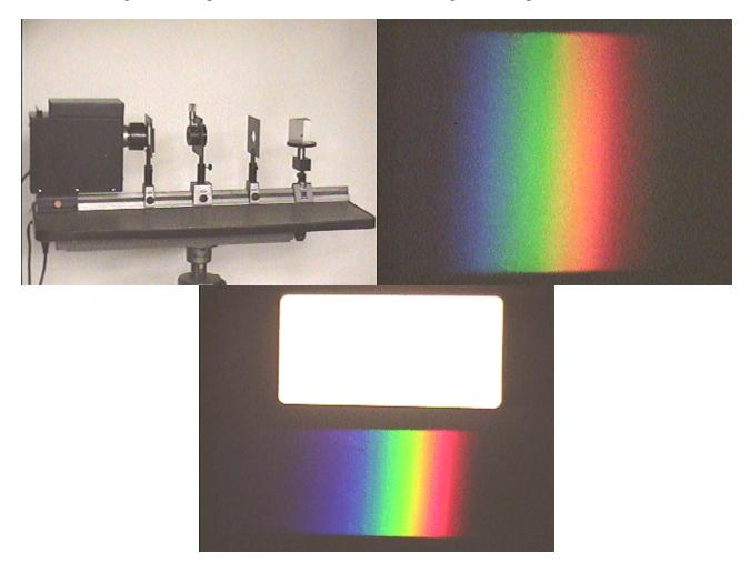
Consider now the light from a high-quality *negative* yellow filter, whose light is seen in the photograph below. The color patch is obtained by placing the filter over a rectangular baffle on an overhead projector. The spectrum is obtained by placing the yellow filter just in front of the slit in the sectrum experiment, as seen in the photograph below the color patch.
