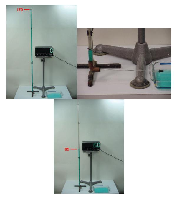
The timer, initially set to zero in the picture at the left, is started at the same time the cap is removed and the water begins to flow out of the tube. The time taken for half of the water to flow out of the tube (the level has gone down from 170 cm to 85 cm) is about 150 seconds, as read on the timer in the photograph at the right.
