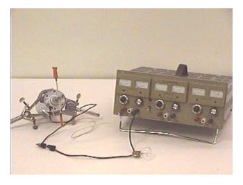
As before, the question is what will happen to the light bulb when the motor and the light bulb are operated in series across the power supply.
