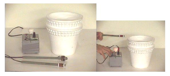
Now the copper coil will be placed into the liquid nitrogen dewar and allowed to cool to the temperature of liquid nitrogen.
