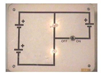
The question this week is: What will happen when the switch is turned ON, closing that part of the circuit circuit?
