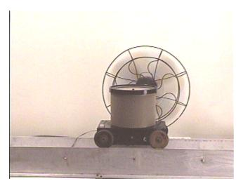
Initially the cylinder is set into motion counterclockwise as seen from above, as can be viewed in a short video by clicking here in <a href="mailto:mpeg">mpeg</a> or <a href="movie">movie</a> format. After the rotor is spinning at full rotational speed, the fan is turned on, blowing air out past the rotor toward the viewer.
