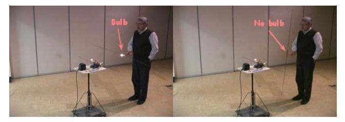
Now suppose that the light bulb is removed from the receiving antenna and it is rotated so that it is vertical, as seen in the photograph at the right.
