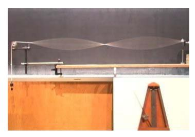
If the waves go by too fast, click <u>here</u> to see the video at a slower speed. Note that there are four wave vibrations for each tick of the metronome.
