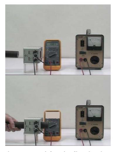
Dan is holding the large iron core, composed of a number of heavy iron wires to mimimize eddy currents, seen in the picture at the left of the coil.
