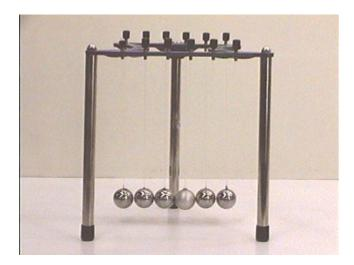
In this case, how will the collision balls apparaus work? In particular, will it work the same way as the equal mass collision ball apparatus? Will the ensuing motion be one ball moving up on one side, then the other side, back and forth?
