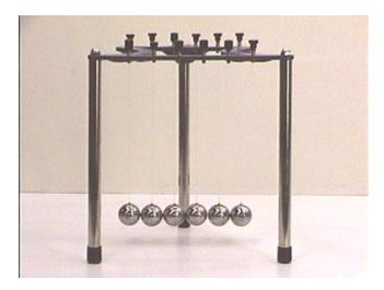
Now suppose that we modify this apparatus, as seen in the photograph below, so that one of the balls (the fourth from the left) is made from aluminum rather than steel, and therefore no longer has the same mass.
