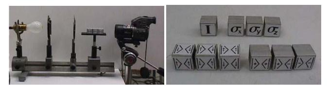
Two little aluminum cubes, seen in the pairs of photographs below, have optical elements in them. If we look through either of the two cubes (right-to-left) with our digital camera, keeping them in the same orientation as in the photograph at the left, the light from the background may be slightly attenuated, but not blocked completely, as seen in the two pairs of photographs directly below.
