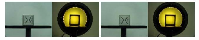
Here are some combinations of two of the above optical elements. Because the color of the light passing through the system is yellow, at this point you may treat *both* the dark green and the black situations as the same: no light is passing through the system.
