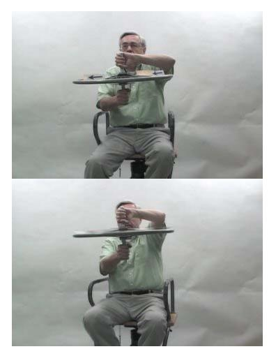
While sitting on the rotating chair, with the rapidly spinning bicycle wheel, I will now turn the wheel upside down, rotating the wheel so that my hands are inverted and the wheel is spinning counterclockwise as seen from above.
