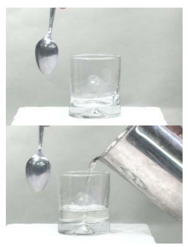
Now suppose that I begin to fill the glass full with water and strike it in the same way, as seen in the photograph at the right above and in an mpeg video by clicking your mouse on the photograph. The video stops just before the glass is about half full.
