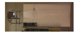
A lens with its surfaces hyperbolic in shape will focus rays from a point object to a point image, as seen in the photograph above and the photograph at the left below.
