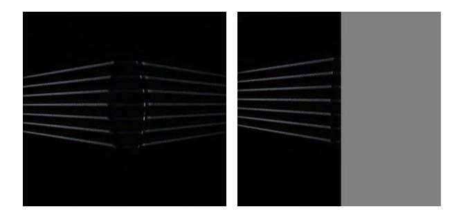
The rays entering and leaving the hyperbolic lens are seen at the left above, and for the segmented lens at the right above. Unfortunately, the right side of the photograph has been masked out, so you cannot see what the rays do after they leave the segmented lens.
