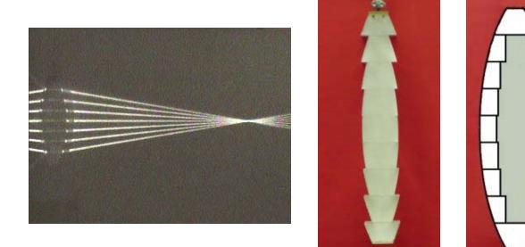
Now suppose that the lens is replaced by the peculiar looking "lens" photographed at the center above. This lens is constructed by removing rectangular segments from the center of the hyperbolic lens and sliding the two outer pieces together to form a sort of "segmented" lens. The figure at the right above shows the outline of the segmented "lens" superposed on the original hyperbolic lens.
