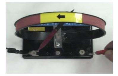
When Dan connects the coil, it might cause the needle to deflect in a different direction, if the field is strong. On the other hand, if the magnetic field of the coil is a different type of field from that of the earth, perhaps nothing will happen. Or maybe the needle will just deflect slightly from where it is with no current in the coil.
