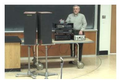
Now suppose that the wires of (ONLY) one of the speakers are reversed, by reversing a toggle switch in the small gray box on the top of the electronics on the cart seen in the photograph. The question here is how that will affect the sound picked up by the microphone in the photograph above.
