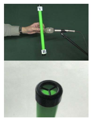
Clicking your mouse on the photograph at the right, you will be able to hear the tone that is produced when the tube is inverted. If end "A" is down, it sounds like an "oo-ah," whereas if end "B" is down it sounds like an "ah-oo."
