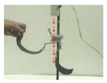
At the top of the photograph is the end of an air blower which, when turned on, will blow air downward onto the convex side of the unrolled sheet. The red arrows show the path of the center of the air stream from the blower past the metal sheet, if the airsteram were to go straight, which may or may not be the case.
