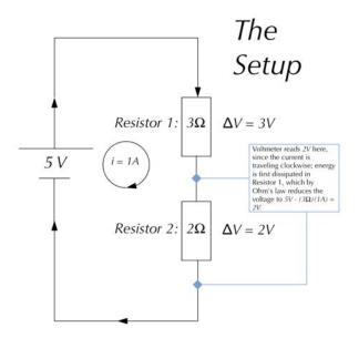
Now, consider the battery reversed, so that current is instead flowing the counter-clockwise direction. Question: What will the voltmeter read now?
