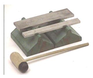
A second gauge block, with the same length and thickness, but twice the width, as seen in the photograph, also produces a tone when struck. The question this week is about the frequency relation between the two tones.
