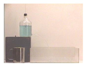
The question involves the range of the water jet - that is, how far away from the bottle the jet shoots by the time it reaches the horizontal level of the top of the container into which the water is squirting. Exactly how does the range of the water jet change as the water level in the jar goes down from the tapered part of the jar to just above the lower end of the capillary tube, where the air is leaving the tube and entering the bottle.
